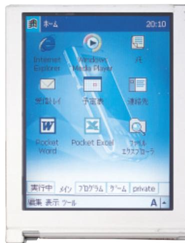
PDA用3.5型QVGA TFT-LCD LTM035A776
