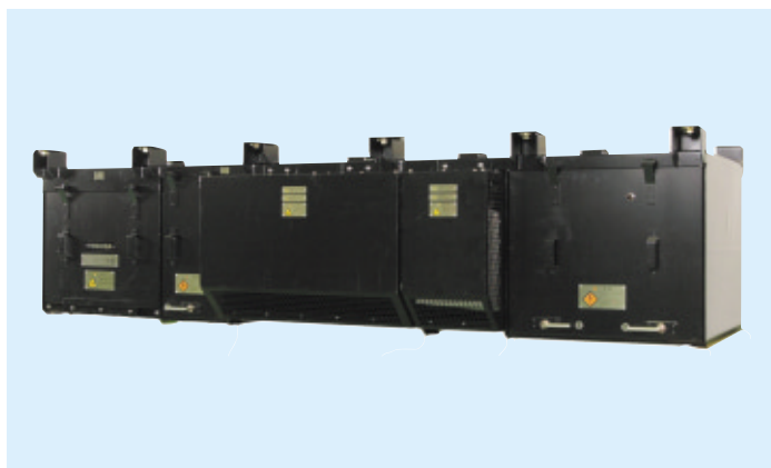
SIV外観 External view of static inverter (SIV)
