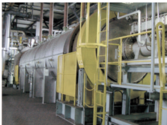
本格稼働した熱分解ガス化炉 Pyrolysis gasification system in full operation
