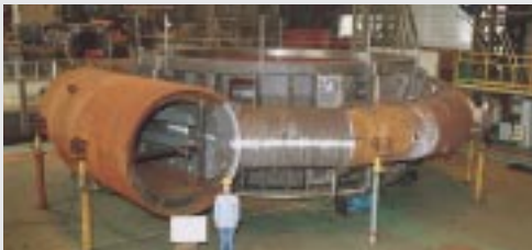
東京電力(株)葛野川発電所向け4号機ポンプ水車の工場組立 Shop assembly of pump-turbine for Kazunogawa Pumped-Storage Power Station Unit No.4 of The Tokyo Electric Power Co., Inc.
