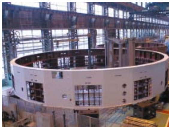
322.2 MVA水車発電機固定子枠 Stator frame of 322.2 MVA hydroelectric generator
