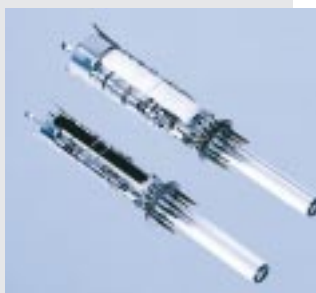
New mini neck electron gun (below) and a conventional electron gun (above)
