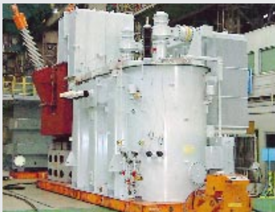
50MVA-110kV gas insulated transformer
