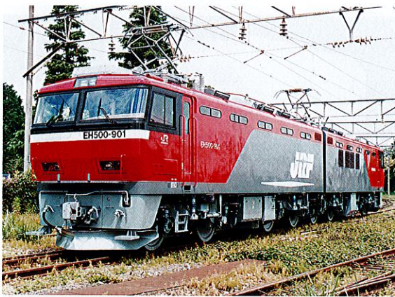
交直流(50/60 Hz)を走破できる EH500 形電気機関車 Series EH500 dual-voltage electric locomotive powered by IGBT
