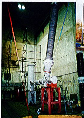
KEMA 形式試験証明書(420 kV GCB)と試験姿 KEMA certificate (420 kV gas circuit breaker short-circuit performance) and outline of KEMA test
