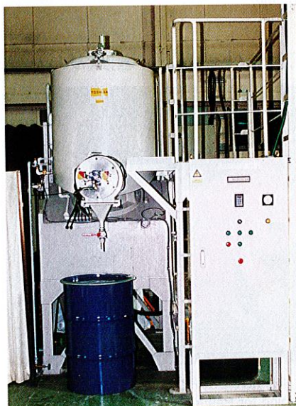
PWR向けセメント固化装置 Cementation system for PWR concentrated waste
