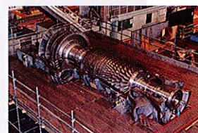
GE-MS7001FA 1,300°C-class gas turbine for Shin-Nagoya Power Station
