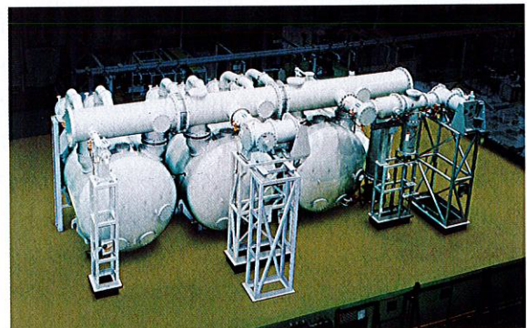
東京電力榊東内幸町変電所納入 275 kV-300 MVA ガス絶縁変圧器 275 kV-300 MVA gas-insulated transformer for Higashi-Uchisaiwaicho Substation of The Tokyo Electric Power Co., Inc.
