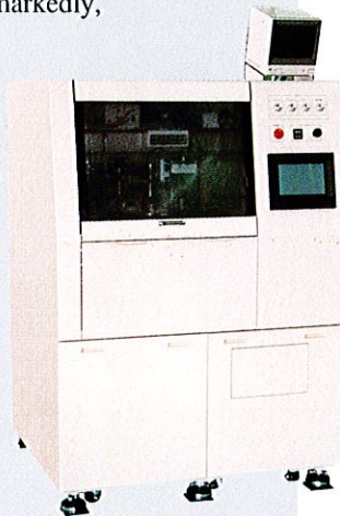
Commercial outer lead bonder for LCDs with a 2 second bonding tact time
