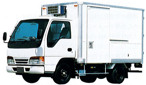
HFC-404A 採用低温用冷凍装置 Low-temperature transport refrigeration unit with HFC-404A refrigerant
