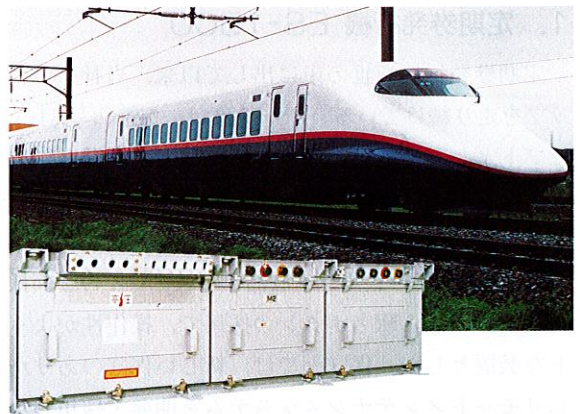
E2系新幹線電車と主変換装置 Series E2 prototype Shinkansen and on-board main converter
