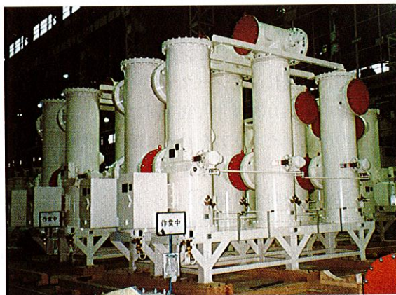
525 kV-40 kA GIS 525 kV-40 kA gas-insulated switchgear
