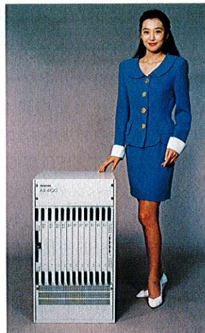
ATM 交換機 AX-4100 AX-4100 ATM private branch exchange
