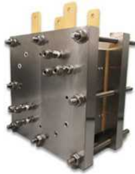
The developed 4-cell stack with an area of 100 cm 2
