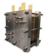
The developed 4-cell stack with an area of 100 cm<sup>2</sup>
