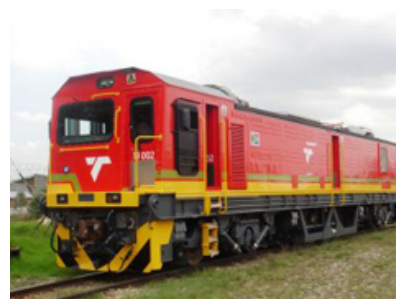
Electric locomotive (15E) for iron ore transport for which Toshiba delivered electric products
