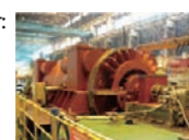
Indirect hydrogen-cooled power generator
