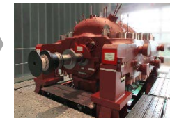
Turbine and combustor for supercritical CO 2 cycle power plant
