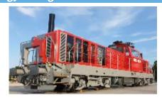
Hybrid locomotive complying with European standards(Drive system combining SCiB™ and PMSM)
