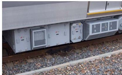
Combined transaction and auxiliary inverter system
