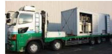
Mobile water treatment system "SARRY-Aqua"
