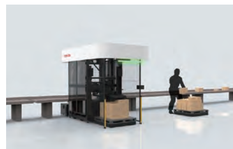
Automatic parcel unloading robot enable to cooperate with humans
