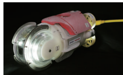
A small robot for investigations inside the nuclear reactor containers (Developed by IRID and Toshiba Energy Systems & Solutions Corp.)
