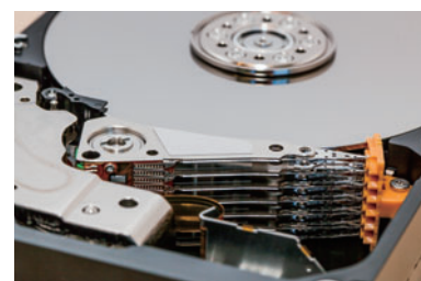
An inside photo of a general HDD with layers of disks and heads for data writing and reading
