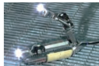
A small-sized robot able to enter and examine the PCV (co-developed by IRID and Toshiba through a government subsidy program for projects of decommissioning and contaminated water management)
