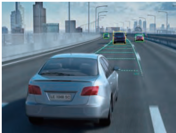
An image recognized by Toshiba image recognition processor, supporting ADAS
