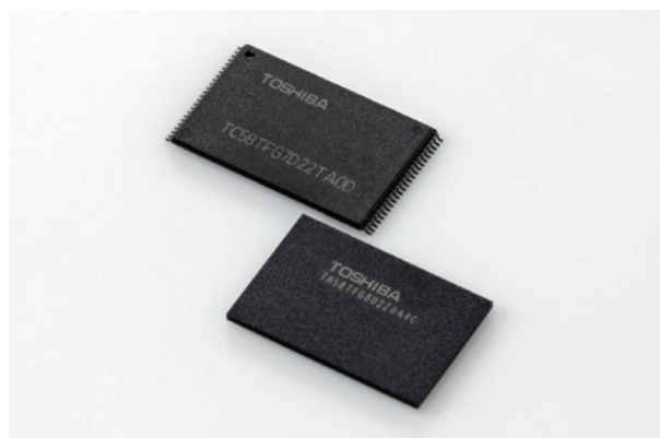
3D flash memory "BiCS FLASH™" based on the world's first 48-layer stacking process
