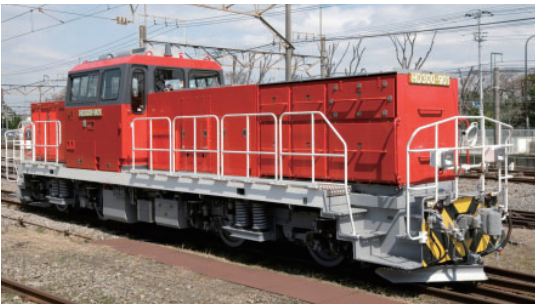
Type HD300 hybrid locomotive (prototype) The "environmentally friendly, clean locomotive," is a hybrid that uses a diesel engine in conjunction with rechargeable battery power; co-developed with Japan Freight Railway Company.
