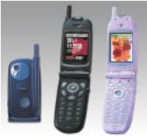
The future of cellular phones: The J-T07 (l.) and TT21 (r.) both have a CCD camera, the A3013T (c.) supports GPS. All three employ a high-resolution low temperature polysilicon TFT LCD.
