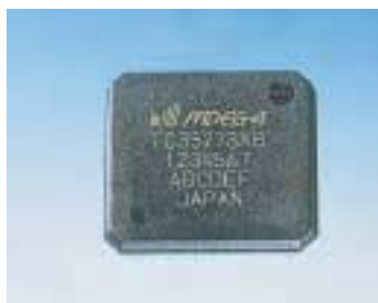
With this LSI, Toshiba will bring MPEG-4 to next-generation cellular phones. Functions include a video phone.
