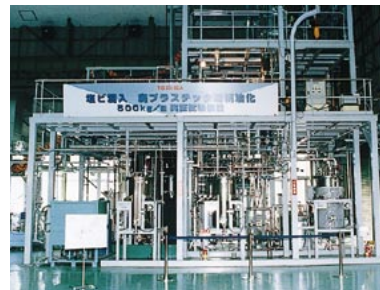
In a major advance, Toshiba discovered a system that transforms used plastics containing up to 50 percent PVC into fuel oil.
