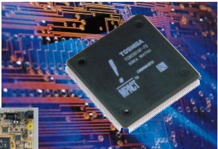
Developed by Toshiba and Chromatic Research, the Mcompact digital signal processor places seven multimedia functions on a single chip.
