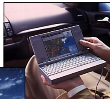
Introduced in Japan in April 1996, the Libretto 20 mini-notebook PC is the world's smallest and lightest PC running Microsoft's Windows 95.
