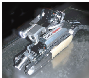
Robot developed by Toshiba and IRID* to survey the insides of nuclear reactor containments
