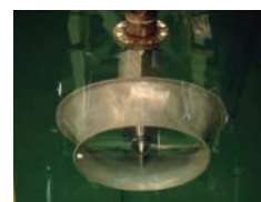
ΣFlow™, a system designed to generate power simply by installing it in a waterway
