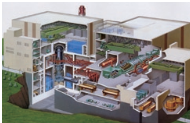
A cross-sectional view of a 1.35-million-kW nuclear power plant
