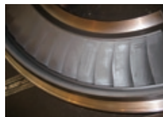
Coating applied to a turbine nozzle
