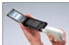
Ultra-compact fuel cell for mobile equipment
