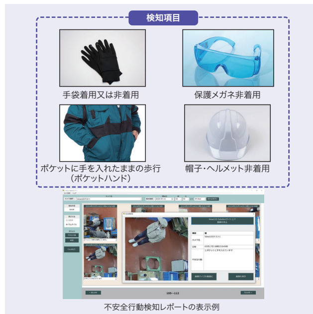
不安全行動検知の概要 Overview of application of ViewLED-based AI image processing in on-premises safety monitoring service
