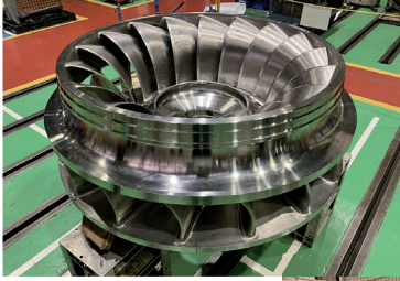
水車ランナ Turbine runner upgrade at Canaveral Hydropower Station, Honduras
