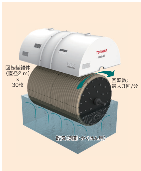
回転繊維体を用いたOD法向け前処理装置 Habuki™ Habuki™ pretreatment system using rotating fiber unit for oxidation ditch
