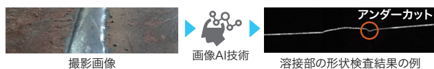
溶接部の3D形状検査 Inspection of three-dimensional shapes of welded parts using AI
