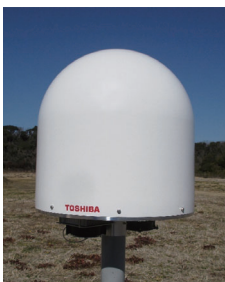
ドローン検知装置試作品 Prototype drone detection system without radio frequency (RF) transmission
