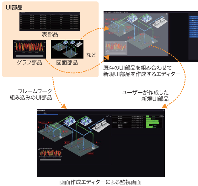
UI部品を組み合わせ設計された監視画面の例 Example of monitoring screen designed with combination of user interface (UI) components
