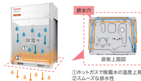
凍結防止対策 Measures to prevent freezing of defrosting water
