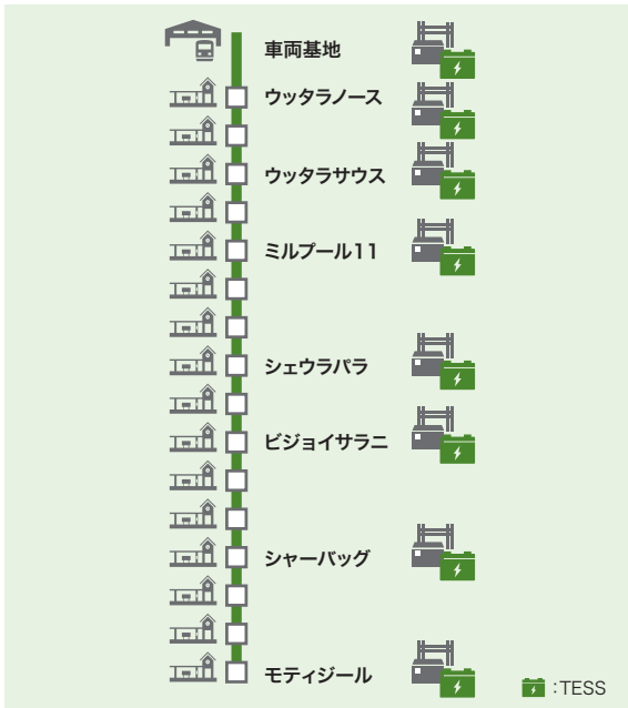
ダッカMRT6号線のTESS設置場所 Locations of traction energy storage systems (TESS) for Dhaka MRT Line 6, Bangladesh
