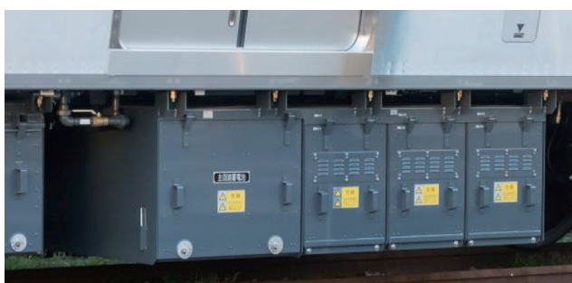
E235系 1000番台車両 非常走行用電源装置の蓄電池 Accumulators of emergency power supply device for E235 1000 series trains of East Japan Railway Company
