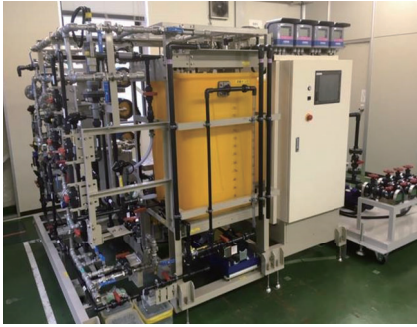
BC膜の実証試験装置 Pilot test equipment for brine concentration (BC) membranes
