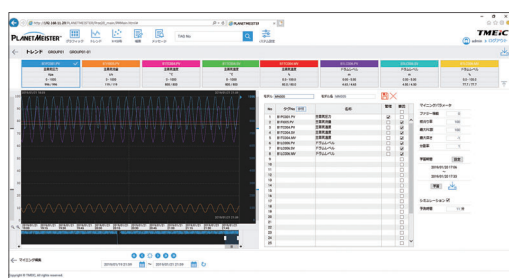
PLANETMEISTER™における品質変動を説明する回帰モデルの構築画面 Example of PLANETMEISTER™ real-time process data management system display to construct regression model elucidating quality variation factors
