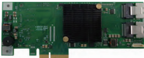
RAIDコントローラー ER383D ER383D redundant array of independent disks (RAID) controller for industrial computers
