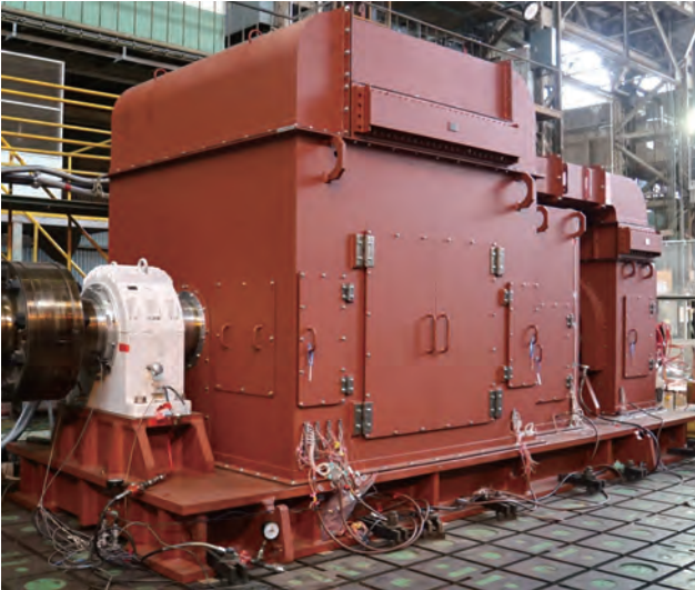
4 極 1,700 MVA 級タービン発電機用ブラシレス励磁装置 Brushless excitation system for 4-pole 1 700 MVA-class turbine generators
