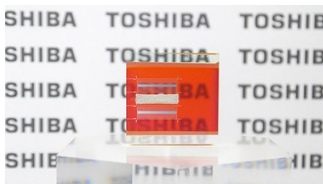
Transparent \text{Cu}_2\text{O} solar cell with PCE of 9.5%
