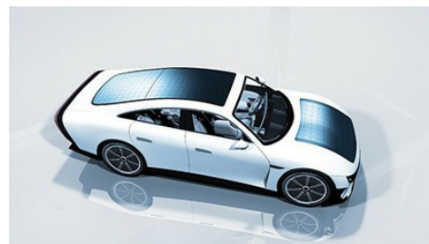
Artist's impression of \text{Cu}_2\text{O} -Si tandem solar cells installed in an EV
