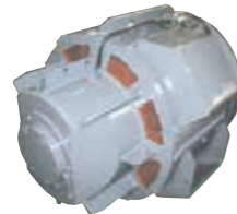
Main alternator for diesel electric locomotive
